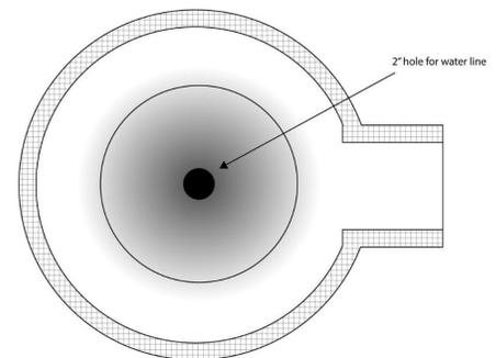
Thread a water line (1\" PVC) from your pool's circulatory system to your scupper bowl. *(If you have chosen to install your water feature on a pillar, you will need to install the line into the middle of the column.)* Your scupper bowl already has a 2\" pre-drilled hole in the center of the basin; thread the line through this hole and add a "tee" fitting to the top of the 1\" PVC. This will help regulate the water flow rate into your bowl.
