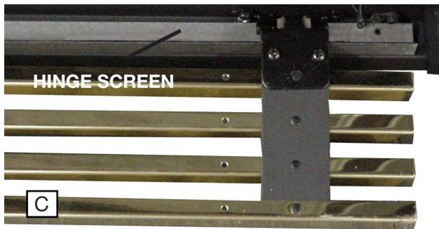
**HINGE SCREEN:** Position the hinge screen into place and with the control door open, secure to the firebox using three screws.
