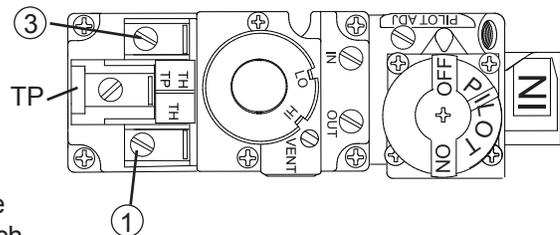
Disconnect the existing wires from terminals 1 and 3 (from the ON/OFF switch) and replace with the leads from the wall switch.
