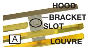
**UPPER LOUVRES:** Insert the upper louvres into the slots on both brackets. Press the top flange of the hood into the four clips located along the top of the appliance as shown.
