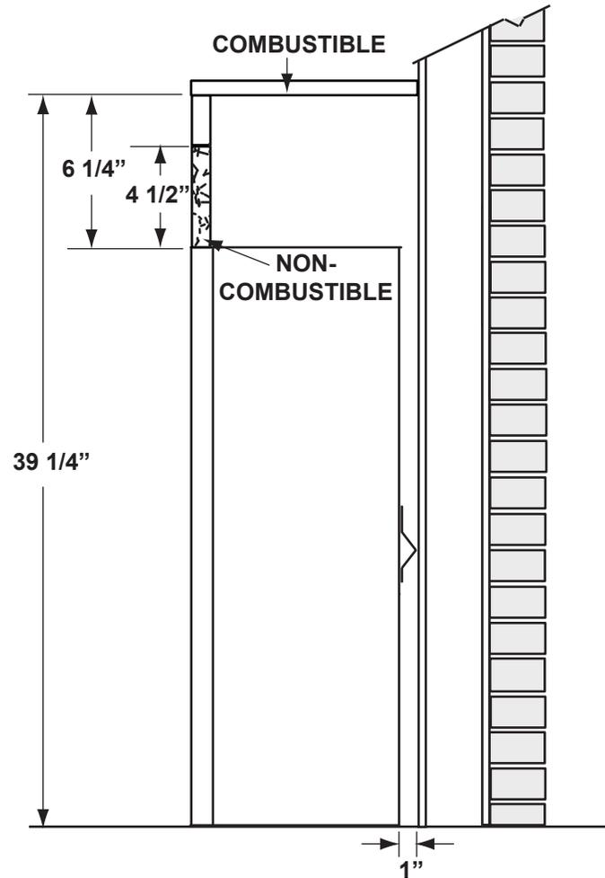
The appliance requires a minimum enclosure height of 39 1/4". For temperature requirements, the enclosure space around and above the appliance must be left unobstructed.
