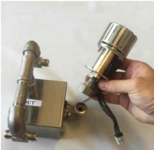
Next, attach the Pilot Burner to the Pilot Burner gas line which is on the side of the box.
