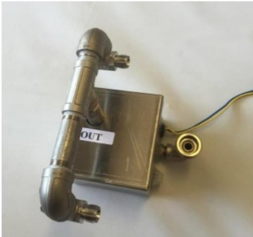
The photo at left shows what this step looks like once complete. Notice the fittings are perpendicular to the sides of the SUBEIS Ignition Control Box.
