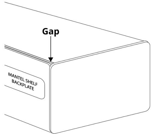
**PLEASE NOTE: It is very easy to scratch the finish during this step. Take precautions to only put stress on the wall-facing lip of the front plate to avoid visible damage.**
