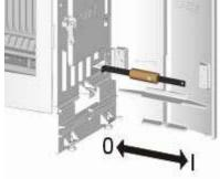
For more accurate control of the burning up of the fuel, an additional combustion air inlet is located underneath the grate, against the rear wall inside the appliance. This inlet can be adjusted with the aid of the
