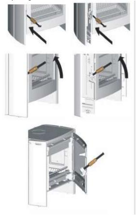
The control handle is inserted horizontally in the centre of the door, in the groove between the left side wall
