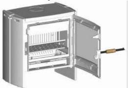
After regular use (depending on the quantity of ash), the grates must be cleaned thoroughly. To do this.
