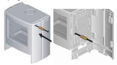
Before the fireplace can be filled via the side filler door, the right side wall must be opened, as described
