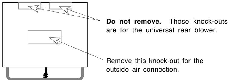
After the precise location of the stove is determined, the outside air boot or pedestal with outside air should be installed prior to installing the stove. Follow the directions included with the outside air boot or pedestal. Make sure to remove the correct knock-out for the outside air option. See the illustration to the left.
