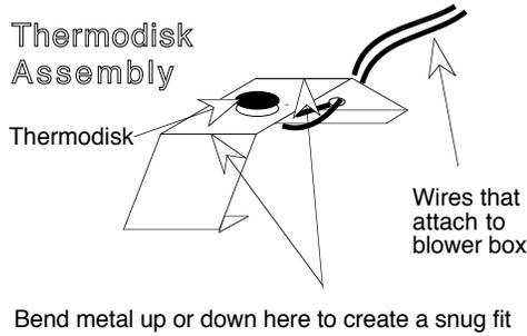
Slide the wire clip over the edge of the strip of metal between the two knock-outs removed in step 1. Insert the two thermodisk wires into the eye of the wire clip and pull the slack wire out of the stove.
