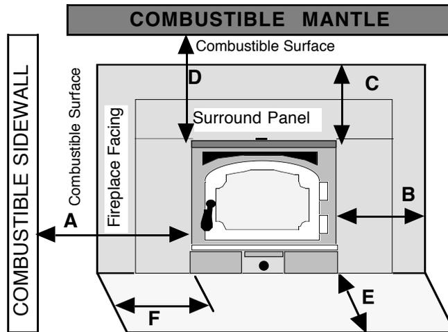
NOTE: For clearances, use this clearance diagram or the clearance diagram on the safety label attached to the back of the appliance.
