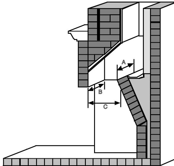
Your template should resemble the drawing on the next page with the dotted lines indicating your initial measurements and the solid line indicating the additional 2". You will use this template to cut a piece of sheet metal (minimum 24 gauge) to install in your smoke chamber.
