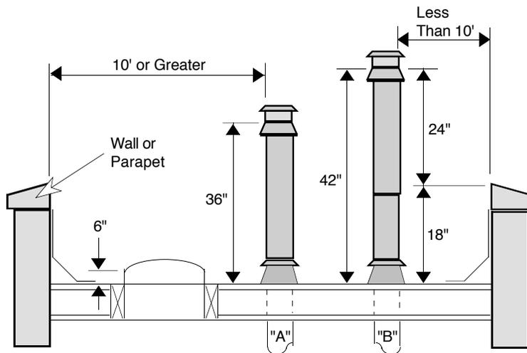
These minimum chimney heights are required by building codes for safety purposes, to allow time for sparks exiting a chimney to cool before they land on the roof. In some problematic situations, additional chimney height above the specified minimums may be necessary to reduce wind-induced down drafting and back puffing, or to increase draft, thereby improving appliance operating characteristics.
