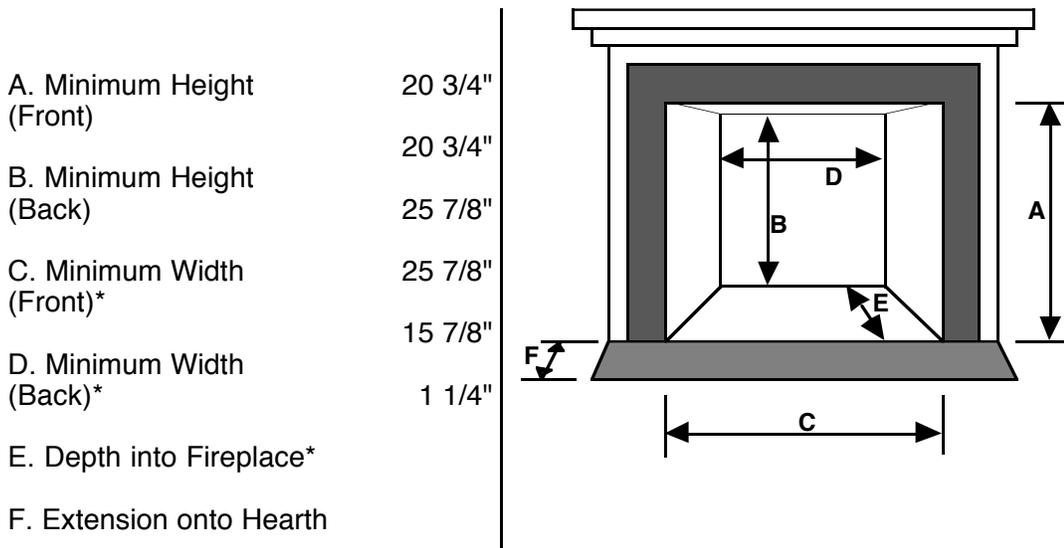
\* These dimensions include the 1" air space required between the sides and back of the insert and the metal firebox of the zero clearance (metal) fireplace.
