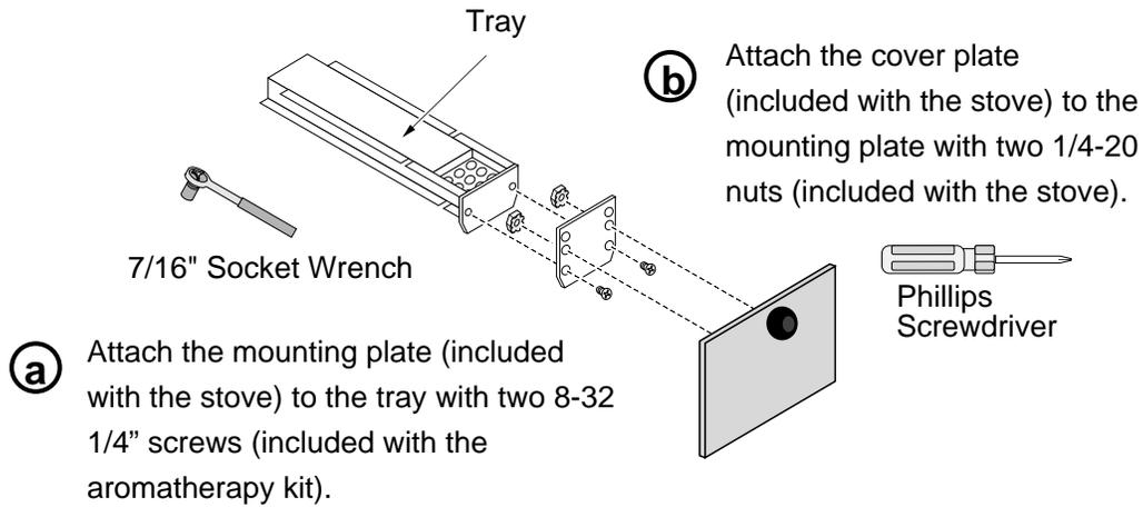
2. Install the extension assembly following the directions below.
