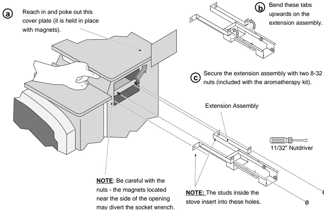
3. Slide the tray into the extension assembly following the directions below.
