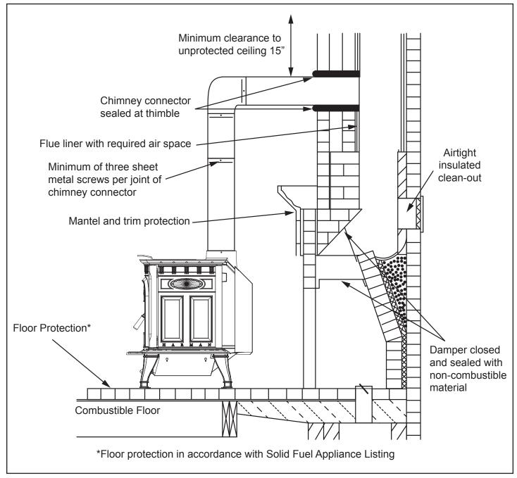
The Chimney Connector Shall Not Pass Through an Attic or Roof Space, Closet or Similar Concealed Space, a Floor or Ceiling.
