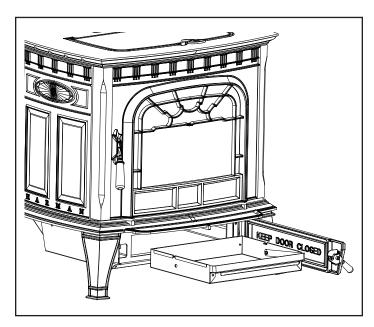
Ashes must be placed in a metal container with a tight fitting lid. The closed container of ashes should be placed on a non-combustible floor or on the ground, well away from all combustible materials, pending final disposal. If the ashes are disposed of by burial in soil or otherwise locally dispersed, they should be retained in the closed container until all cinders have thoroughly cooled. Do not use the ash container for other debris or yard waste.
