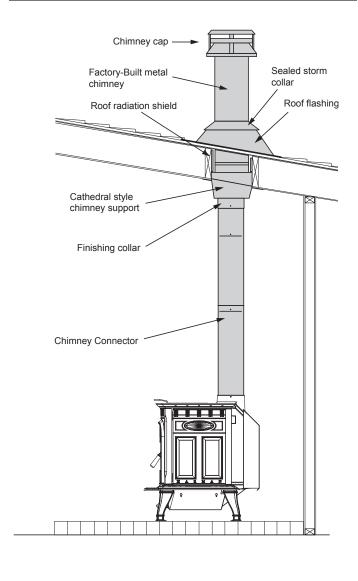
The Chimney Connector Shall Not Pass Through an Attic or Roof Space, Closet or Similar Concealed Space, a Floor or Ceiling.
