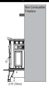
If the fireplace floor can hold the 500 lb. (250 kg) Oakwood, the stove should only be placed into the fireplace opening to the point that operation of the damper bypass control and the top load door operation is not compromised or unsafe. (See above illustration.)
