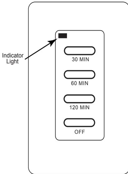
The wall timer operates on a (2) 3V button cell batteries (included) made specifically for remote controls and electronic lighters. Before using the wall transmitter, install the two (2) 3V button cell batteries. Follow the instructions below.
