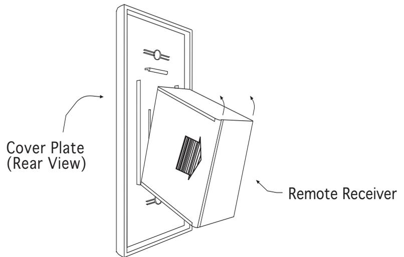
Position the cover plate so the word ON is facing up; then, install the remote receiver into the plastic switch box using the two long screws provided. Push the White Button over the receiver slide switch only after making sure the remote receiver has LEARNED the transmitter's security code (see LEARNING TRANSMITTER TO RECEIVER) section.
