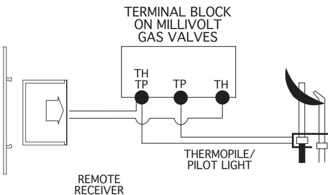
Operation of the remote receiver is similar to that of a thermostat in that both turn the gas valve ON and OFF based on input signals. A thermostat's input signals are different temperatures. The remote receiver's input signals come from the transmitter.
