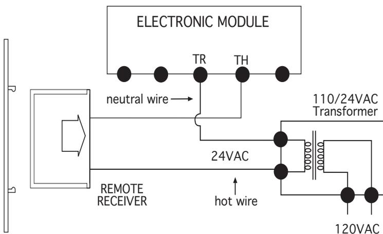
The remote control receiver can be connected, in series between a 24VAC transformer and the TR terminal on the ELECTRONIC MODULE. Connect the hot wire from the 24VAC transformer to either of the wire on the remote receiver. Connect another wire (included) between the other receiver wire terminal and the TH (thermostat) terminal on the ELECTRONIC MODULE.
