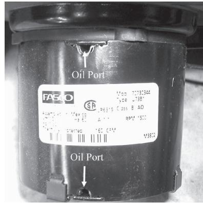
Figure 24. Holes for screws on the right side panel. Figure 25. Oil ports on a circulation fan.
