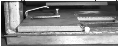
BYPASS DOOR REMOVAL THROUGH COMBUSTOR OPENING
