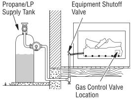
Figure 16 - Checking Gas Joints (Propane/LP Model Shown)
