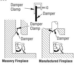
Figure 10 - Attaching Damper Clamp
