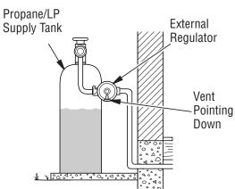
Figure 13 - External Regulator With Vent Pointing Down
