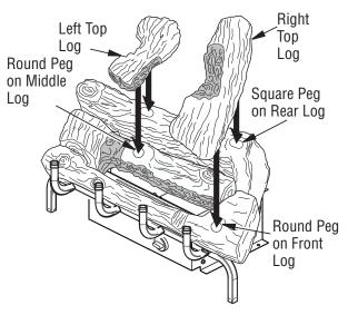
Figure 23 - Installing Left and Right Logs (Picture may vary from actual)
