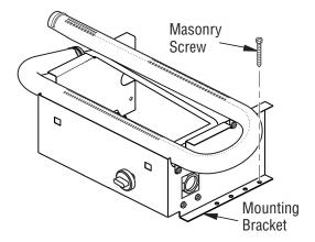
Figure 12 - Attaching Base to Fireplace Floor
