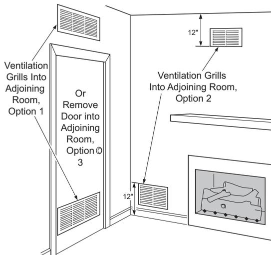
**Figure 2 - Ventilation Air from Inside Building**
