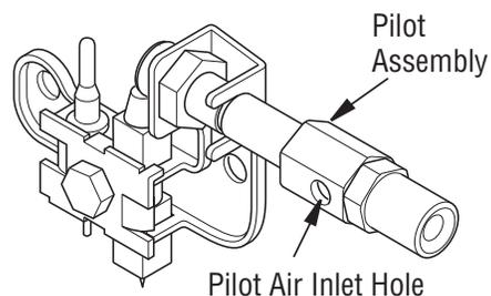
**Figure 43 - Pilot Inlet Air Hole**
