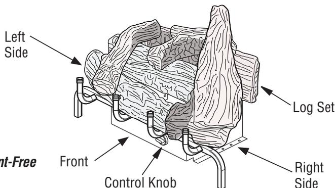
**Figure 1 - Yellow Flame Vent-Free Gas Log Heater**
