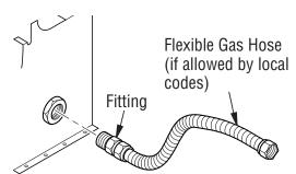
Figure 11 - Attaching Flexible Gas Hose to Heater
