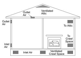
Figure 3 - Ventilation Air from Outdoors
