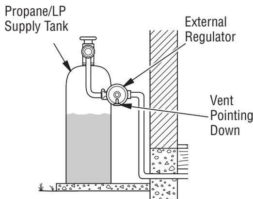
**Figure 13 - External Regulator With Vent Pointing Down**
