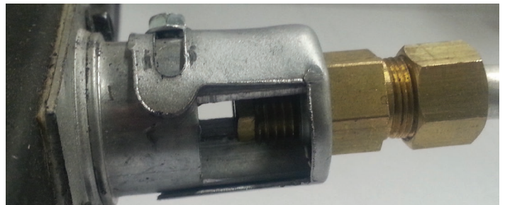
Figure 3 - Air Shutter Fully Open
