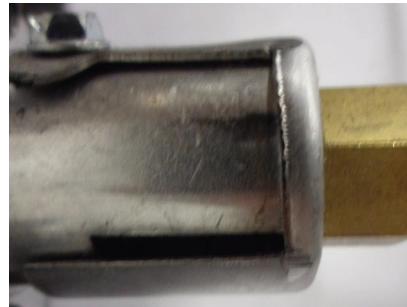
Figure 1 - Air shutter at 1/8-inch opening
