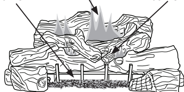
Figure 46 - Incorrect Burner Flame Pattern
