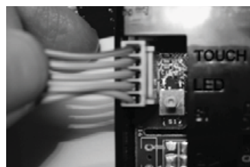
Figure 20 - Connecting end of Touch Pad Cable
