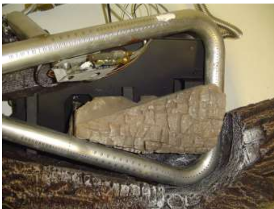
Figure 27A - Installing Charred Log Top View
