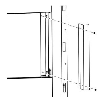
Figure 21 - Installing Side Face Filler for See-Thru Applications
