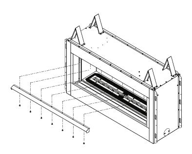
Figure 15 - Installing Hood
