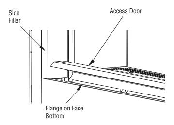
Figure 22 - Access Door for See-Thru Applications
