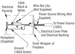
Figure 7 - Connecting Electricity
