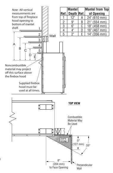
Figure 5 - Clearances for Combustible Mantels
