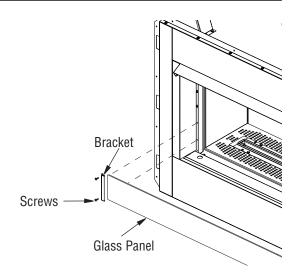
Figure 25a - Installing Draft Shield Kit
