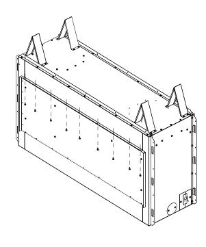
Figure 16 - Removing Rear Panel for See-Thru Applications
