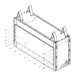
Figure 14 - Installing Rear Panel for Regular Applications
