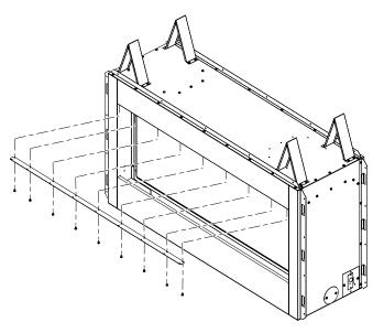
Figure 17 - Removing for See-Thru Applications
