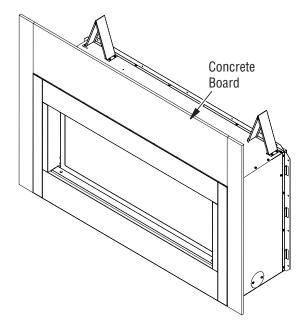
Figure 4 - Installing Concrete Board
