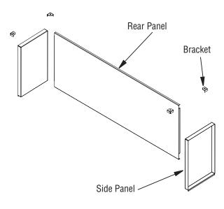
Figure 19 - Removing Rear Interior Wall for See-Thru Applications
