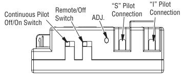
Figure 26 - Gas Module Right Side
