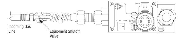
Figure 29 - Turning Equipment Shutoff Valve to the OFF Position
