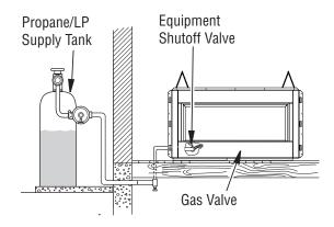
Figure 12 - Checking Gas Joints for Propane/LP Gas Fireplace
