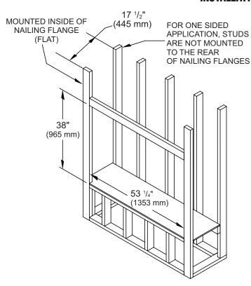
Figure 2 - Framing Clearances for One Sided Application
