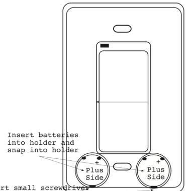
Insert small screwdriver into slot and pop-out batteries from holder
