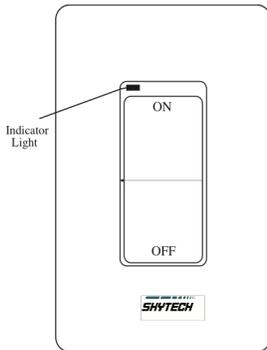
The wall transmitter operates on a (2) 3-volt button cell batteries (included) made specifically for remote controls and electronic lighters. Before using the wall transmitter, install the two (2) 3-volt button cell batteries. Follow instructions below.
