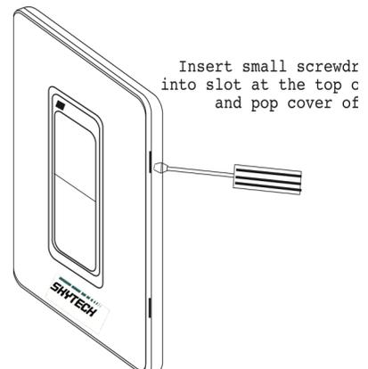
Insert small screwdriver into slot at the top and pop cover of
