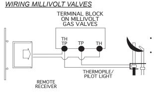
Connect one wire from the remote receiver to the TH terminal on the gas valve.
