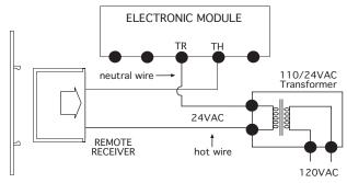
The remote control receiver can be connected, in series, to a 24VAC transformer to the TR (transformer) terminal on the ELECTRONIC MODULE. Connect the hot wire from the 24VAC transformer to either of the wire terminals on the remote receiver. Connect another wire between the other receiver wire terminal and the TH (thermostat) terminal on the ELECTRONIC MODULE.
