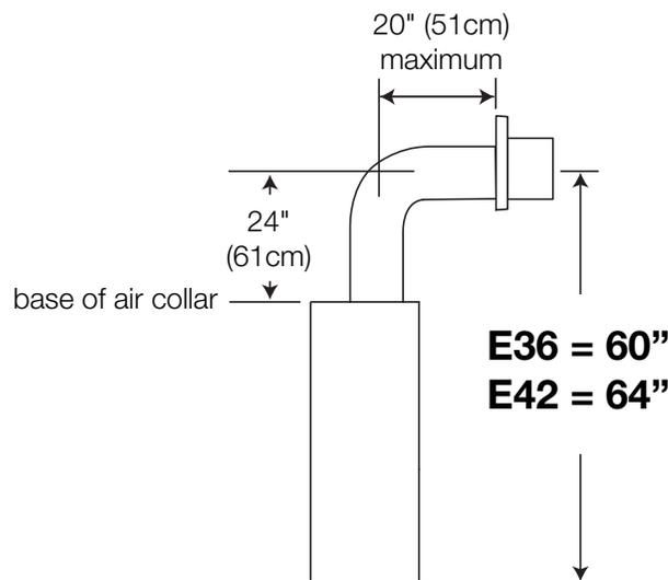
Use the periscope kit to locate the air termination above grade. The periscope must be installed so that when final grading is completed, the bottom air slot is located a minimum 12" (30.5cm) above grade. The maximum allowable vent length is 10' (3m) for a fireplace and 8' (2m) for a stove.
