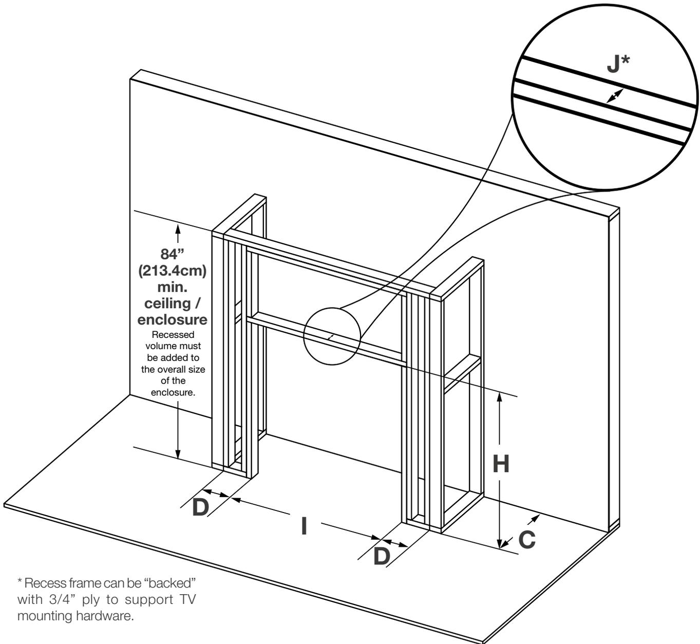
\* Recess frame can be "backed" with 3/4" ply to support TV mounting hardware.
