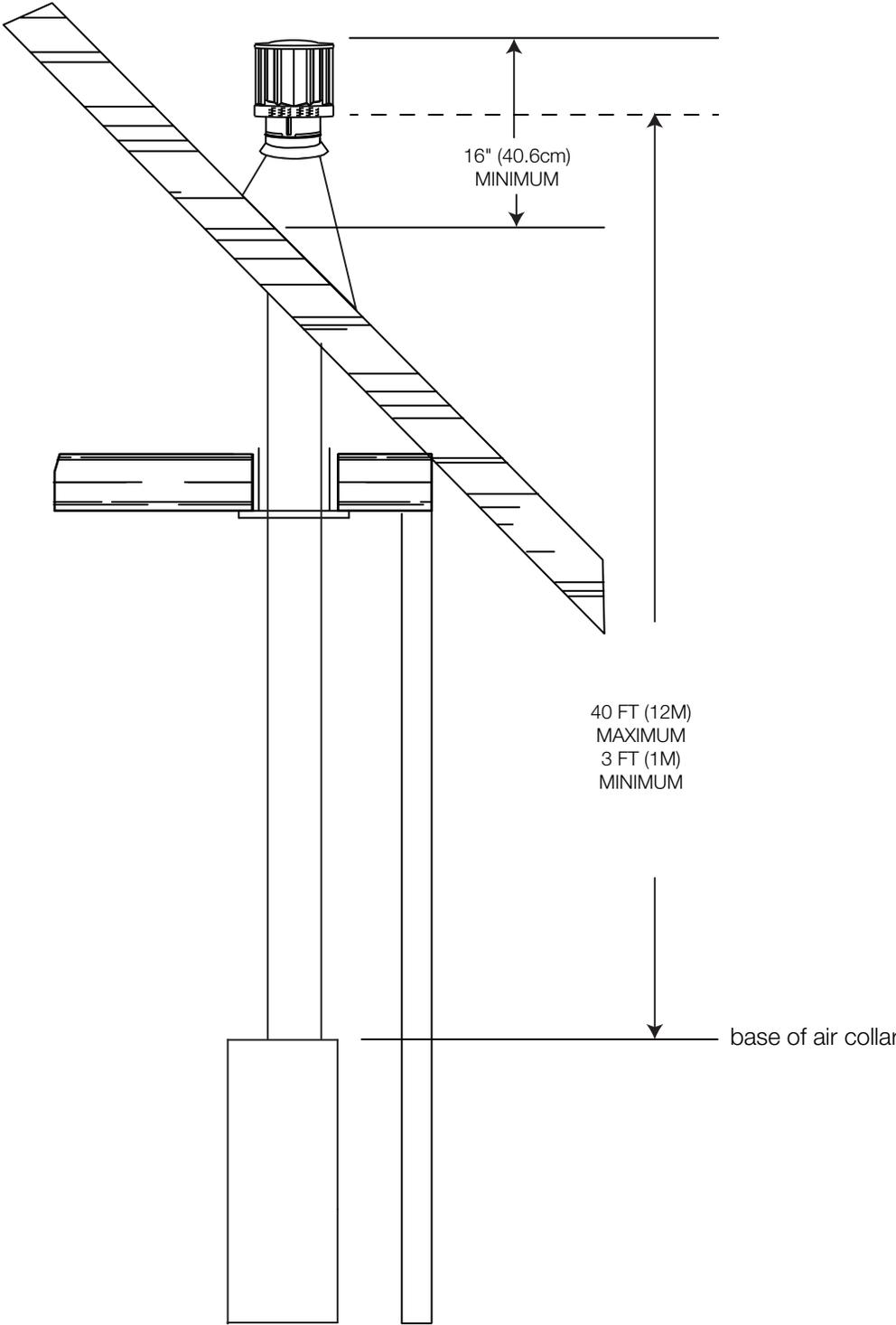
\* Refer to "venting requirements" and "venting installation" sections.
