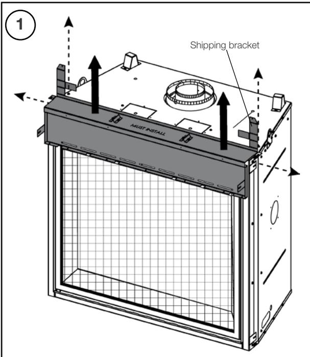
Remove the 4 screws securing the header shield. Remove the shipping brackets by breaking them off or folding them out of the way.
