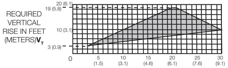
HORIZONTAL VENT RUN PLUS OFFSET IN FEET (METERS)  $H_T$
