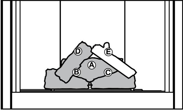
E. Place the right crossover log (W135-0579) onto the two remaining pins.
