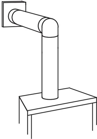
See graph to determine the required vertical rise  $V_T$  for the required horizontal run  $H_T$ .
