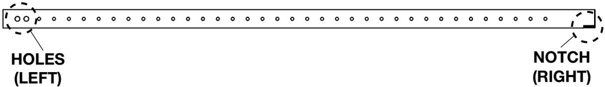
1. With the appliance door open or removed, insert the left side of the secondary air tube into the hole in the **left side** of the appliance.
