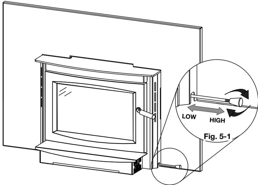
Inadequate draft may cause back-puffing into the room through the appliance and chimney connector points and may cause plugging of the chimney. Too much draft may cause an excessive temperature in the appliance, glowing red appliance parts or chimney connectors or an uncontrollable burn which can lead to a chimney fire or permanent damage to the appliance.
