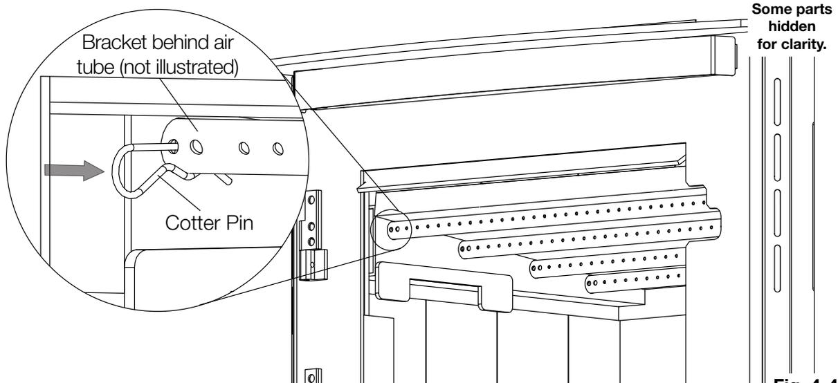
4. Spread the cotter pin to retain the secondary air tube in place.
