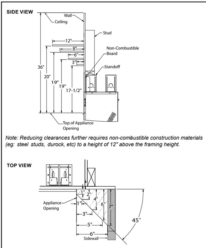
**Back Wall Clearance** — The appliance may be placed against a combustible back wall.
