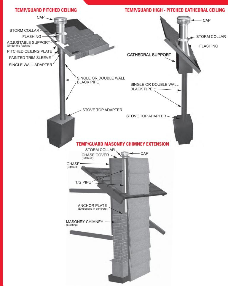
Note: Twist Lock Pipe (6"-12") overlaps  $1\frac{1}{2}$ " when joined together. Quick Connect Lock (14"-18") overlaps  $1\frac{1}{2}$ " when joined together with sheet metal screws. Therefore, assembled length on all sizes is  $1\frac{1}{2}$ " less than listed length.
