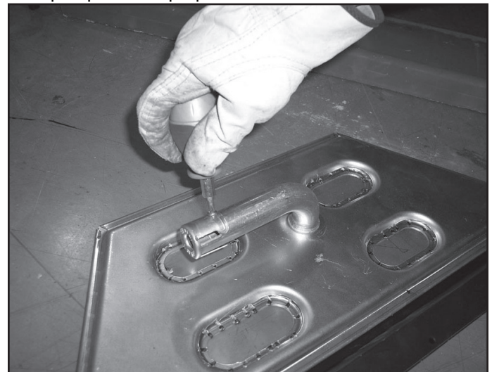
Figure 14.31 Adjust Air Shutter
