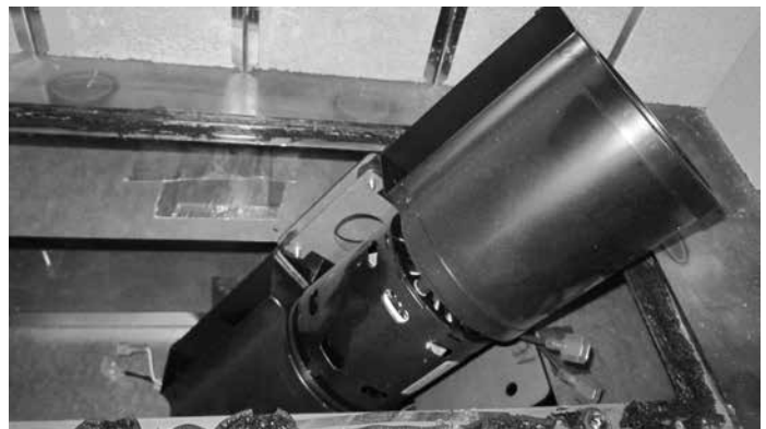
Figure 4.14 Remove Fan from Access Hole
