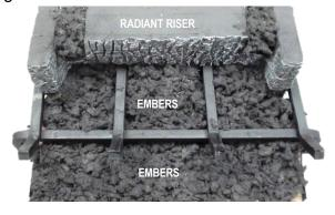
STEP 4: Stuff the embers into the notches of the Radiant Riser and cover all visible burner media as shown in figure 4. Now install the Radiant Heat series logs according to the log diagram sheet included with you log set.
