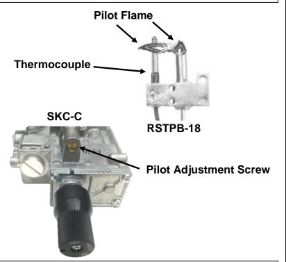
**IMPORTANT:** These controls are factory preset and will not normally require additional adjustment of the pilot flame. If field adjustment of the pilot flame is required, adjust using the pilot adjustment screw. The 90 degree pilot should produce 2 flames about  $1-1 \frac{1}{2}$ " in 2 directions. One flame should come towards the front of the firebox to ignite the burner and the other, wrapping around the thermocouple to ensure proper valve operation.
