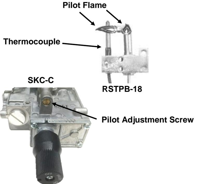
**IMPORTANT:** These controls are factory preset and will not normally require additional adjustment of the pilot flame. If field adjustment of the pilot flame is required, adjust using the pilot adjustment screw. The 90 degree pilot should produce 2 flames about 1-1 1/2" in 2 directions. One flame should come towards the front of the firebox to ignite the burner and the other, wrapping around the thermocouple to ensure proper valve operation.
