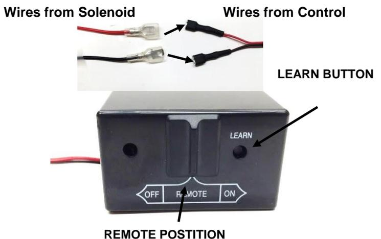
**IMPORTANT:** It is recommended that the remote control box be installed outside the firebox to insure maximum durability during its operation. For application in which the control box is located in the firebox use Fiber Heat Shield (FRCHSCL) to protect the control box.
