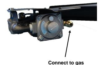
**IMPORTANT:** The minimum inlet supply pressure for the purpose of input adjustment is 5.0 inches (natural gas) 11 inches (propane gas) in water column. The maximum inlet supply pressure is 10.5 inches (natural gas) 13 inches (propane gas) in water column.
