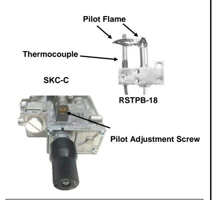
IMPORTANT: These controls are factory preset and will not normally require additional adjustment of the pilot flame. If field adjustment of the pilot flame is required, adjust using the pilot adjustment screw. The 90 degree pilot should produce 2 flames about 1-1 ½" in 2 directions. One flame should come towards the front of the firebox to ignite the burner and the other, wrapping around the thermocouple to ensure proper valve operation.
