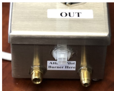
Pilot Burner Gas Valve Outlets (Brass) (Blow Compressed Air in through Outlets)
