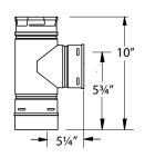
Attaches 3" pipe to branch and 4" pipe to body. Use for a  $90^{\circ}$ offset. Branch swivels for alignment. Removable twist-lock Clean-Out Tee Cap.
