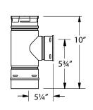
Use for a 90° offset. Branch swivels for alignment. Removable twist-lock Clean-Out Tee Cap.
