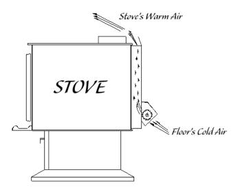
You can also install the quick connect thermodisc kit, included with your stove, to enable the blower to start or stop automatically when the stove is hot or too cold.
