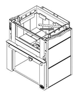
1- Starting with the rear tube, lean and insert the right end of the secondary air tube into the rear right channel hole. Then lift and insert the left end of the tube into the rear left channel.
