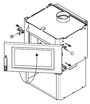
Remove the latch (M) and reinstall the screws (L) that were securing the assembly into the holes.
