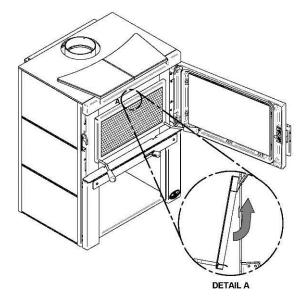
Lean the upper part of the fire screen against the top door opening making sure to insert the top fire screen brackets behind the primary air deflector as in (Detail A).
