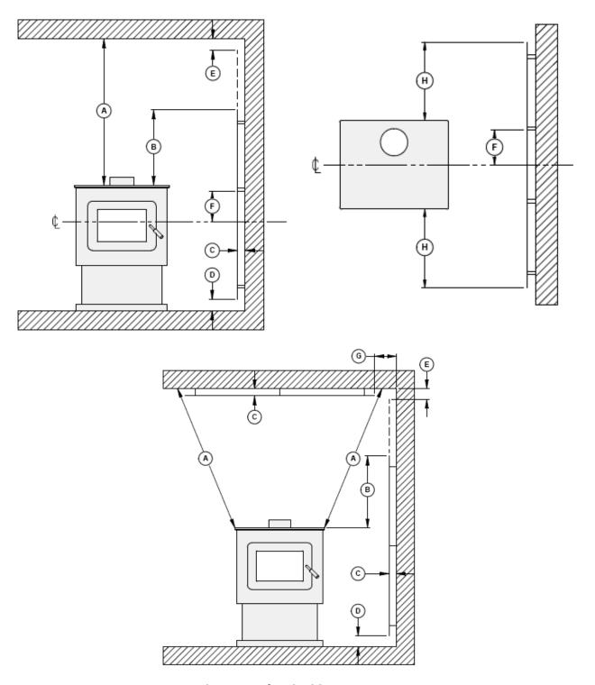
**Clearances for shield construction**
