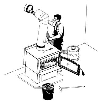
**CAUTION:** Operation of your stove without the baffle may cause unsafe and hazardous temperature conditions and will void the warranty. **NOTE:** Before installing the firebrick, check to ensure that none are broken or damaged in any way. If so, have the damaged ones replaced. Check the firebrick for damage at least annually and replace any broken or damaged ones with new ones. Inspection and cleaning of the chimney is facilitated by the removable baffle.
