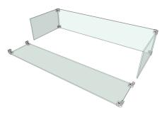
**4.** Now that you've connected the three pieces together, turn it over so that it is upright. Now grab the sole remaining piece and connect it to the rest of the unit.
