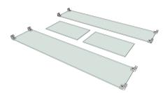
**2.** To begin, attach the corner connectors onto the longer pieces of glass. Tighten the connectors with a screw driver. Do not over-tighten, damage may occur.
