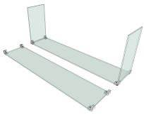
**3.** On one piece, attach the shorter pieces of glass to create a "U" shape. Tighten the connectors.
