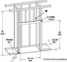
**Rough Framing Face** (dimension includes finish material inside framing, if any)
