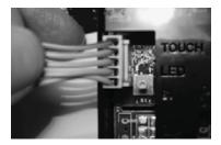
Figure 27 - Connecting end of Touch Pad Cable
