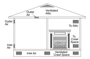
Figure 4 - Ventilation Air from Outdoors
