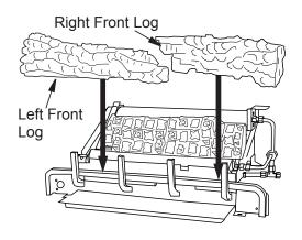
Figure 29 - Installing Left/Right Front Logs
