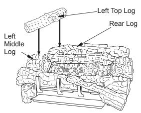
Figure 36 - Installing Left Top Log
