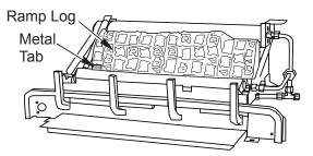
Figure 28 - Installing Fiber Ramp Log
