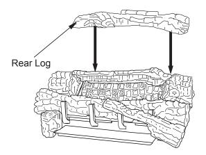
Figure 35 - Installing Rear Log
