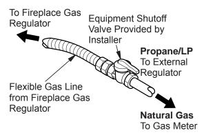
Figure 20 - Attaching Flexible Gas Lines Together
