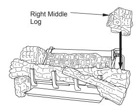
Figure 33 - Installing Right Middle Log
