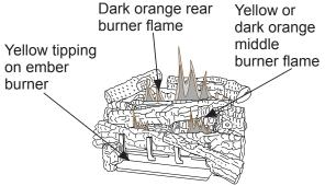
Figure 49 - Incorrect Burner Flame Pattern
