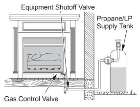
Figure 23 - Checking Gas Joints for Propane/LP Gas
