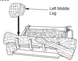
Figure 32 - Installing Left Middle Log
