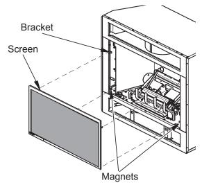
Figure 42 - Installing Fireplace Screen
