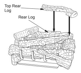
Figure 38 - Installing Top Rear Log
