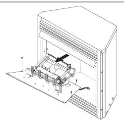
Figure 19 - Removing Log Base Assembly From Fireplace
