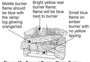
Figure 48 - Correct Burner Flame Pattern
