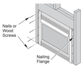
Figure 15 - Attaching Fireplace to Wall Studs
