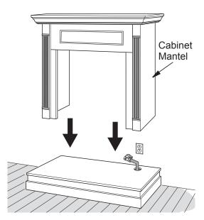
Figure 10 - Installing Cabinet Mantel
