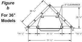
Figure 14 - Rough Opening for Installing in Corner
