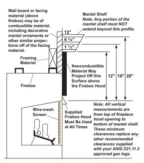
Figure 16 - Minimum Mantel Clearances for Built-In Installation
