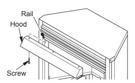
Figure 5 - Installing Hood
