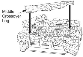
Figure 37 - Installing Middle Crossover Log
