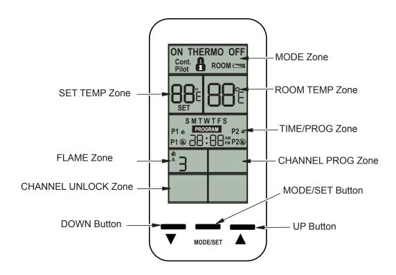
Figure 43 - Touch-Screen LCD and Button Layout
