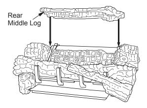
Figure 34 - Installing Rear Middle Log
