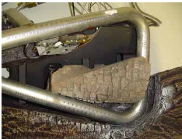
Figure 21A - Installing Charred Log Top View
