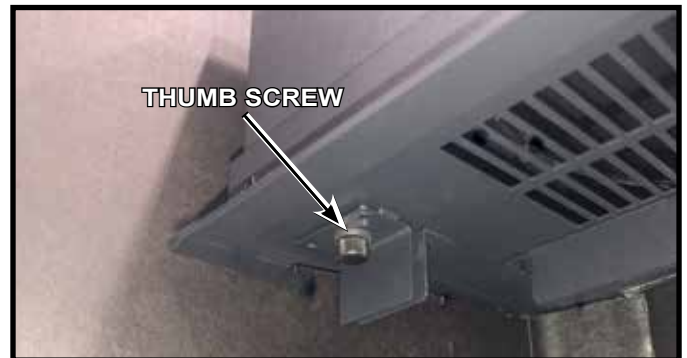
Figure 4.16 Glass Removal and Installation
