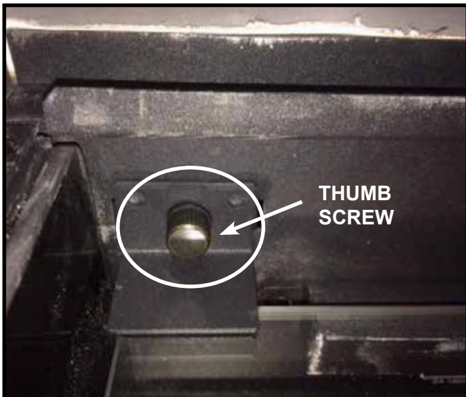
Figure 4.12 Glass Removal and Installation
