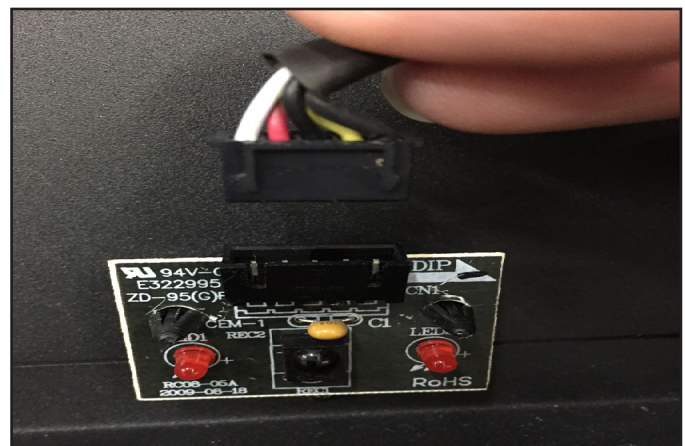
Figure 12 Disconnect Wiring Harness from Remote Receiver Board
