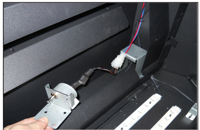
Figure 18 Electrical Connection required for replacement for the Faux Flame Motor.
