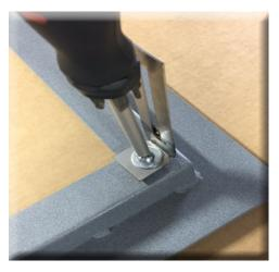
**2.** Attach mounting brackets on all four corners as shown. Use washer & small screw.
