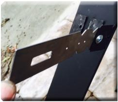
3. With bolt, washer and nut (included) attach install tabs as shown.
