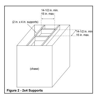
If you are unable to put supports under the chase top to support the cap (as shown in Figure 2), we suggest using two pieces of aluminum angle (1/2 inch x 3/4 inch).
