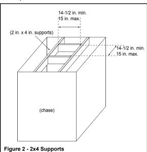
If you are unable to put supports under the chase top to support the cap (as shown in Figure 2), we suggest using two pieces of aluminum angle (1/2 inch x 3/4 inch).
