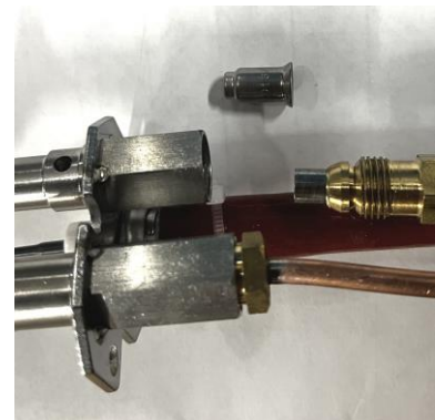
Figure 9.3 – Cleaning pilot orifice
