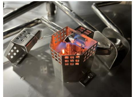
Figure 9.2 – Pilot flame coverage of thermocouple.
