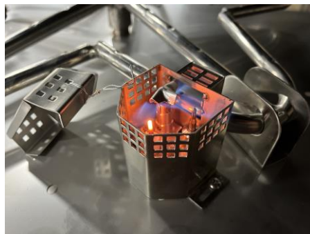
Figure 9.2 – Pilot flame coverage of thermocouple.
