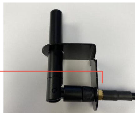
Figure 6.6 – Attach antenna cable
