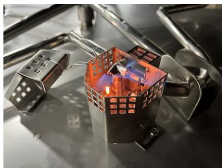
Figure 9.2 – Pilot flame coverage of thermocouple.
