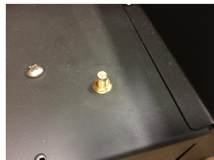
Figure 6.7 – Attach antenna cable
