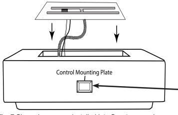
Fig. 7 Shows burner pan installed into Sanctuary enclosure.
