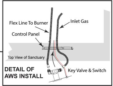
Fig. 8 Shows TPSI system installing into enclosure.
